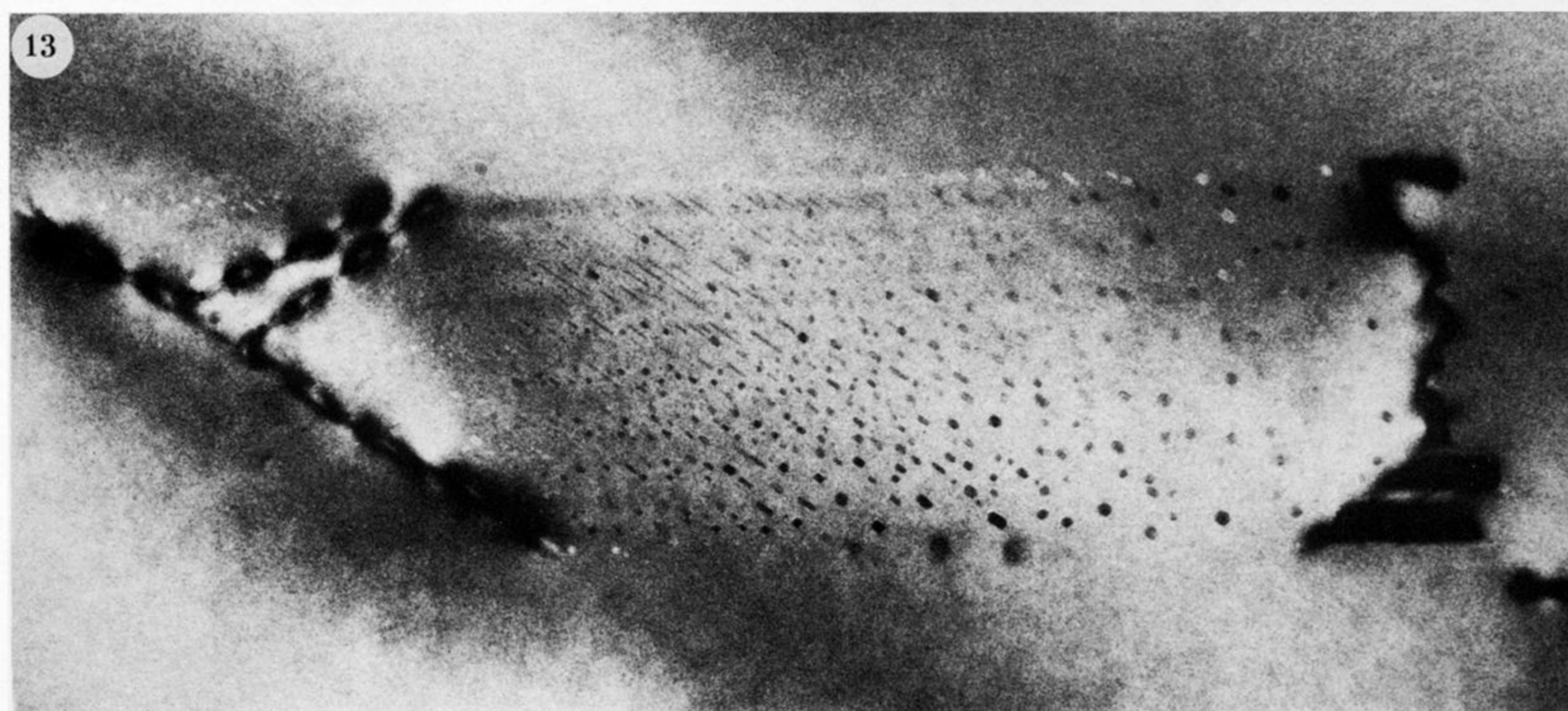
FIGURE 13. Partial platelet with high ratio of voidite sheet area to platelet area in the image. Highly elongated voidites appear in upper part of image of voidite sheet. Width of partial platelet image is 0.9\ \mu\text{m} , specimen thickness is 0.23\text{--}0.25\ \mu\text{m} (7532, original magnification \times 4 \times 10^4 ).
