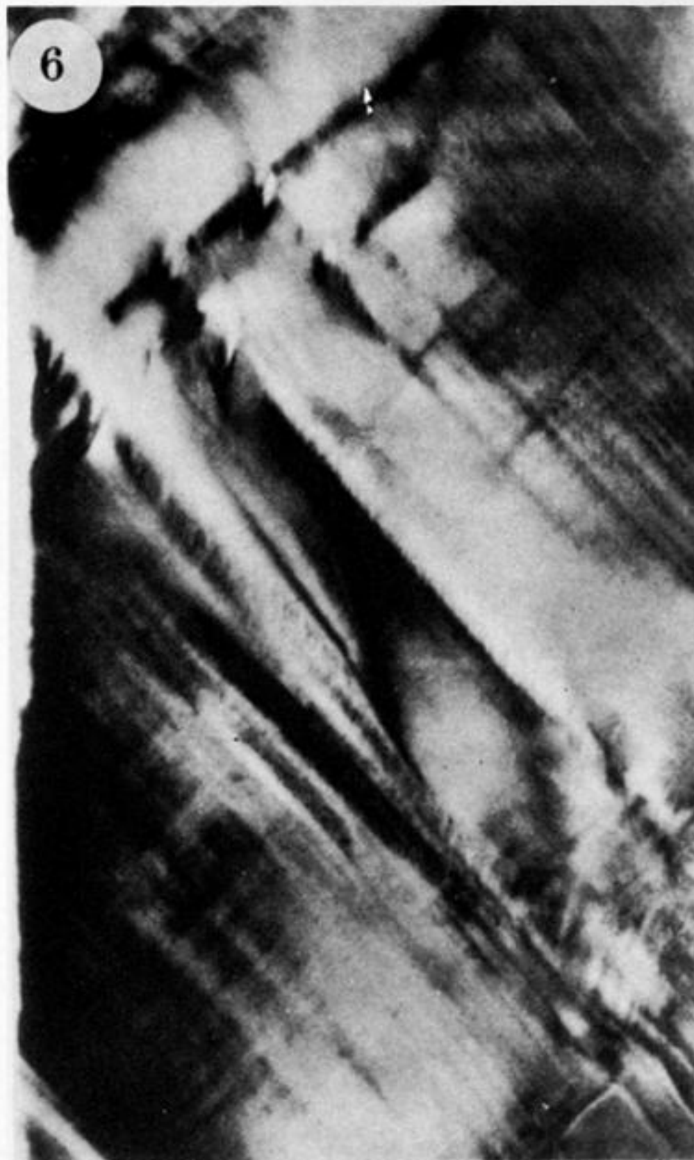
FIGURE 6. X-ray section topograph through specimen DL4 showing intersecting \{111\} slip traces. Height of section 2 mm. Direction [00\bar{1}] vertical. Bragg reflection 2\bar{2}0 obtained in symmetrical transmission through 1 mm thick specimen, projection of diffraction vector points to the right. Cu K\alpha_1 radiation, Bragg angle 37.6^\circ .
