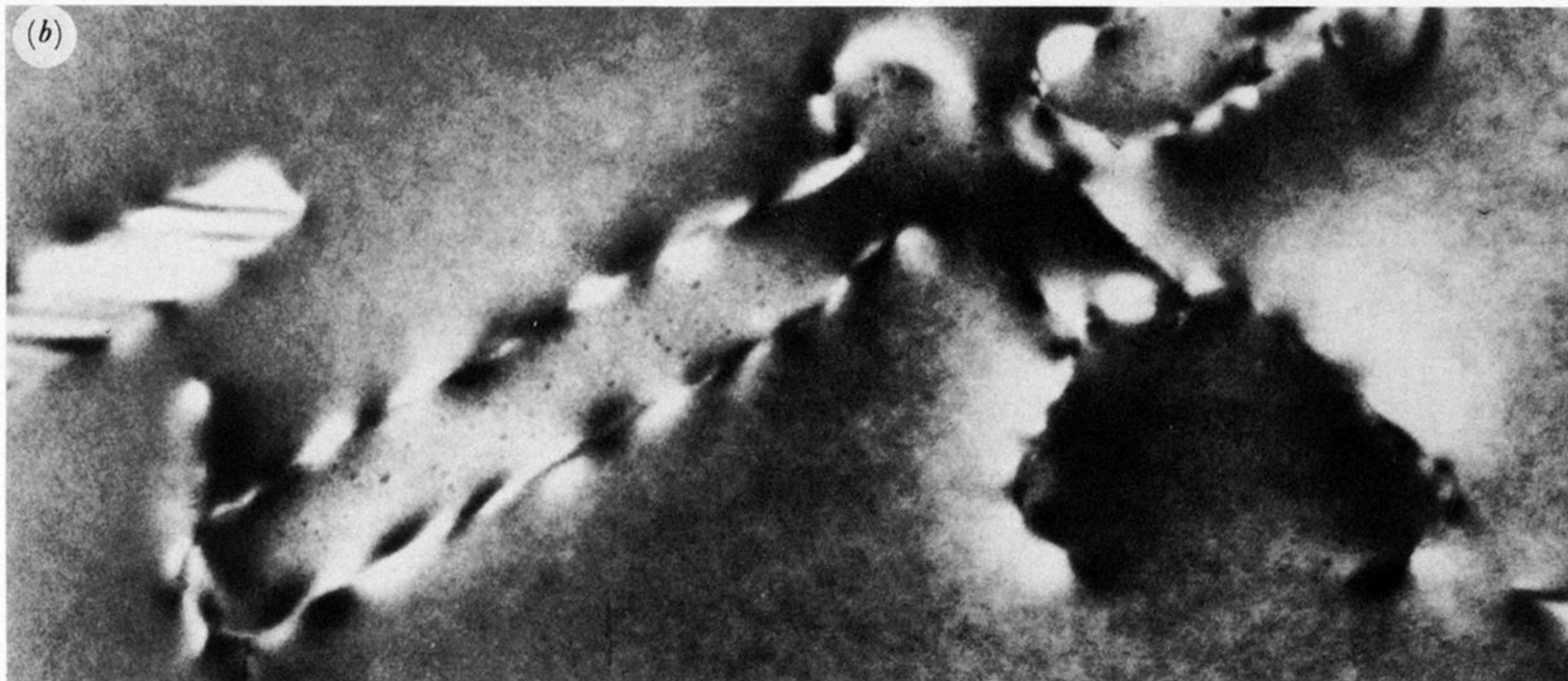
FIGURE 20. Voidite-containing dislocation loops. Direction [001] is horizontal, field width is 0.8 \mu\text{m} . Comparison of (a) bright-field (4706, original magnification \times 6 \times 10^4 ), and (b) dark-field image, 111-type reflection (4707).
