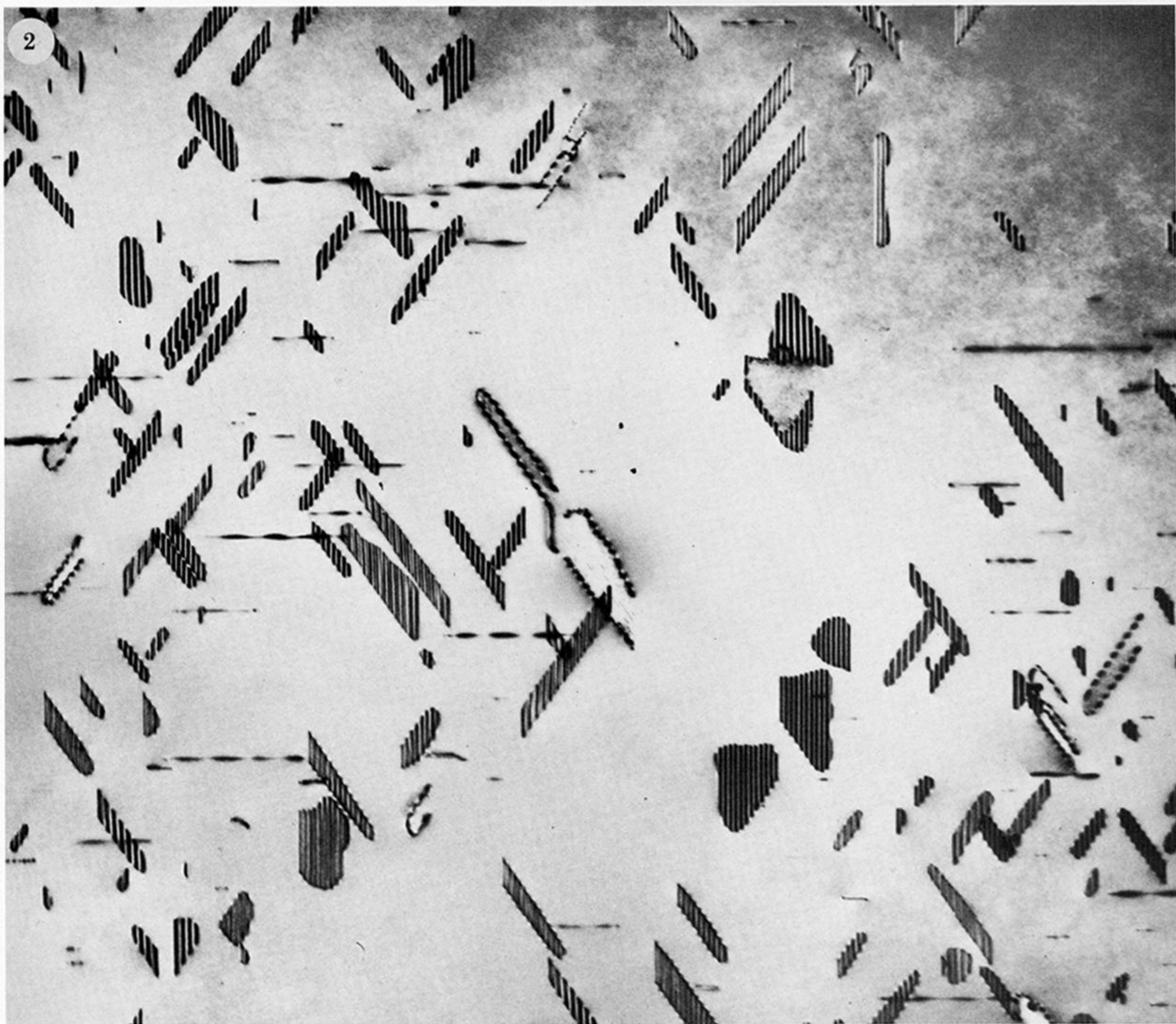
FIGURE 2. A zone in specimen A4 containing large platelets and voidite-containing dislocation loops. One annular partial platelet also appears. Specimen thickness in centre of field is 0.3\ \mu\text{m} . Electron accelerating voltage 120 kV. In this figure and in figures 4 and 8, [001] points towards top of field and the field width is 4\ \mu\text{m} (8071, original magnification \times 10500 ).
