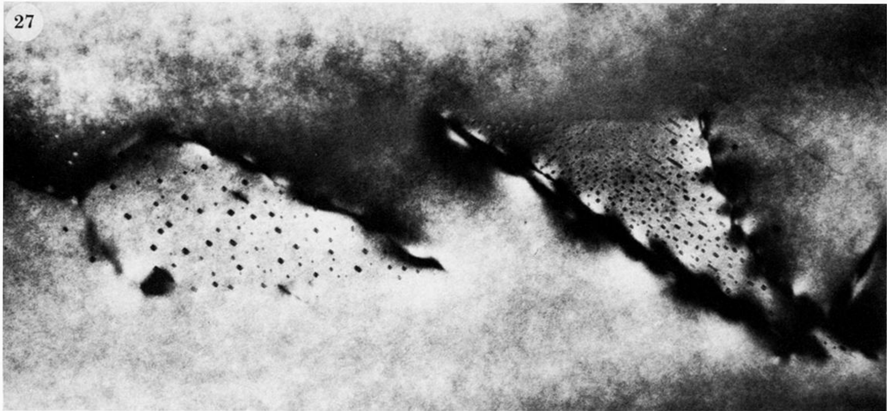
FIGURE 27. Pair of voidite sheets. Evidence of residual fault surface contrast appears along the outcrop of the right-hand voidite sheet. Direction [001] is horizontal, field width is 0.9\ \mu\text{m} (J6971, original magnification \times 6 \times 10^4 ).
