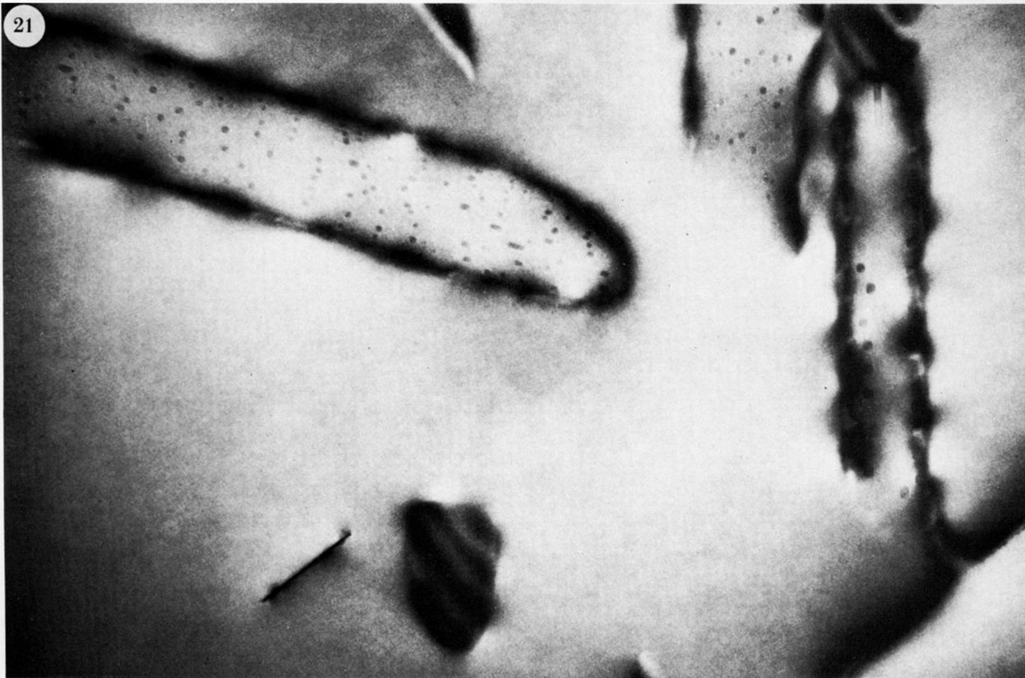
FIGURE 21. Group of voidite-containing dislocation loops with some platelets. Direction [001] rotated 52^\circ clockwise from horizontal. Field width is 0.5 \mu\text{m} (4723, original magnification \times 1.5 \times 10^5 ).
