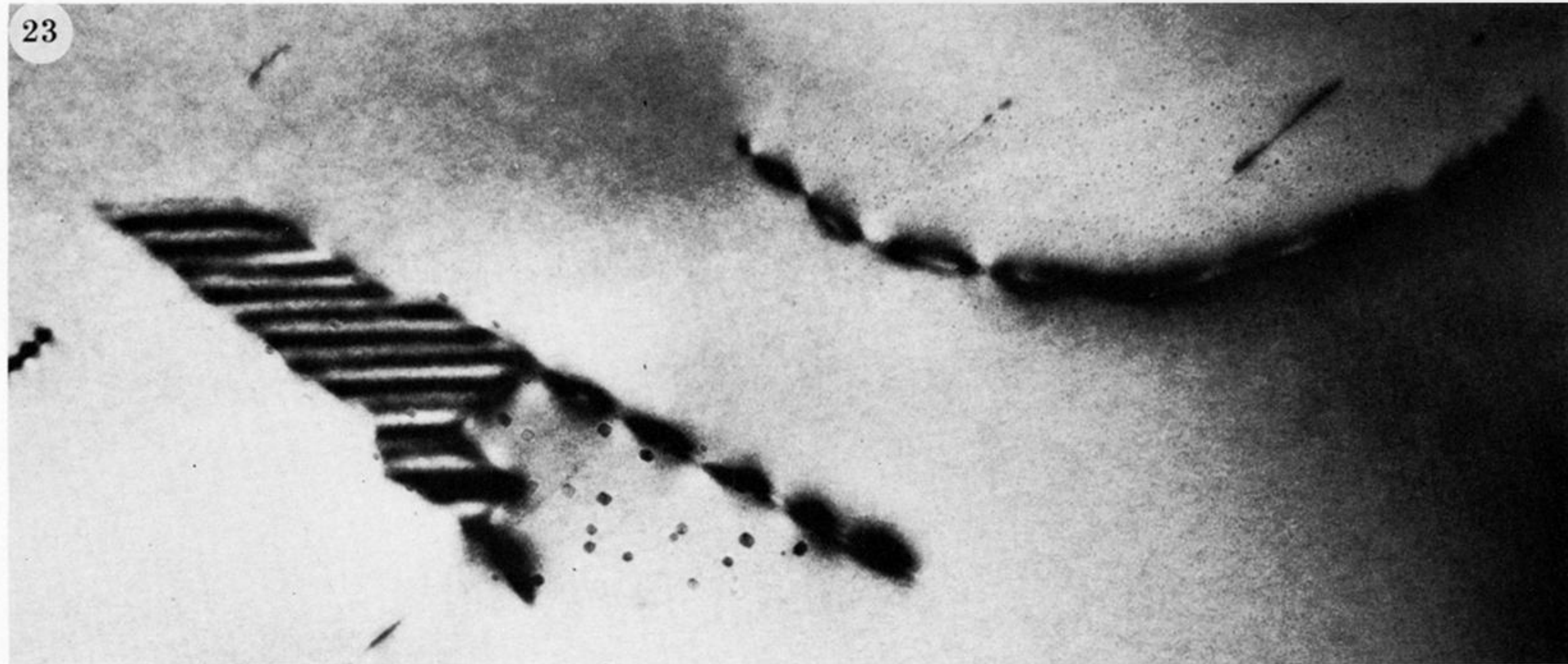
FIGURE 23. Partial platelet (left) with voidites on the platelet area, and a dislocation loop segment (upper right) containing many small voidites with diameters < 1 \mu\text{m} . Direction [001] rotated 5^\circ anticlockwise from horizontal. Field width is 1 \mu\text{m} and specimen thickness is 0.25 \mu\text{m} (G6949, original magnification \times 4 \times 10^4 ).
