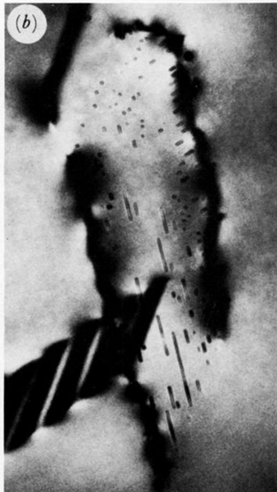
FIGURE 3. Detail in the large voidite-containing loop at the centre of the field of figure 2. The image is rotated about 17^\circ clockwise relative to figure 2 (magnification \times 160000 ). (a) Enlargement from the low-magnification micrograph, figure 2. (b) High magnification and resolution, electron accelerating voltage 200 kV, close to optimum focus. Longest voidite image is about 3 \times 80 nm in projection. (4709, original magnification \times 10^5 .) (c) As (b), but underfocused by about 1 \mu\text{m} (4716).
