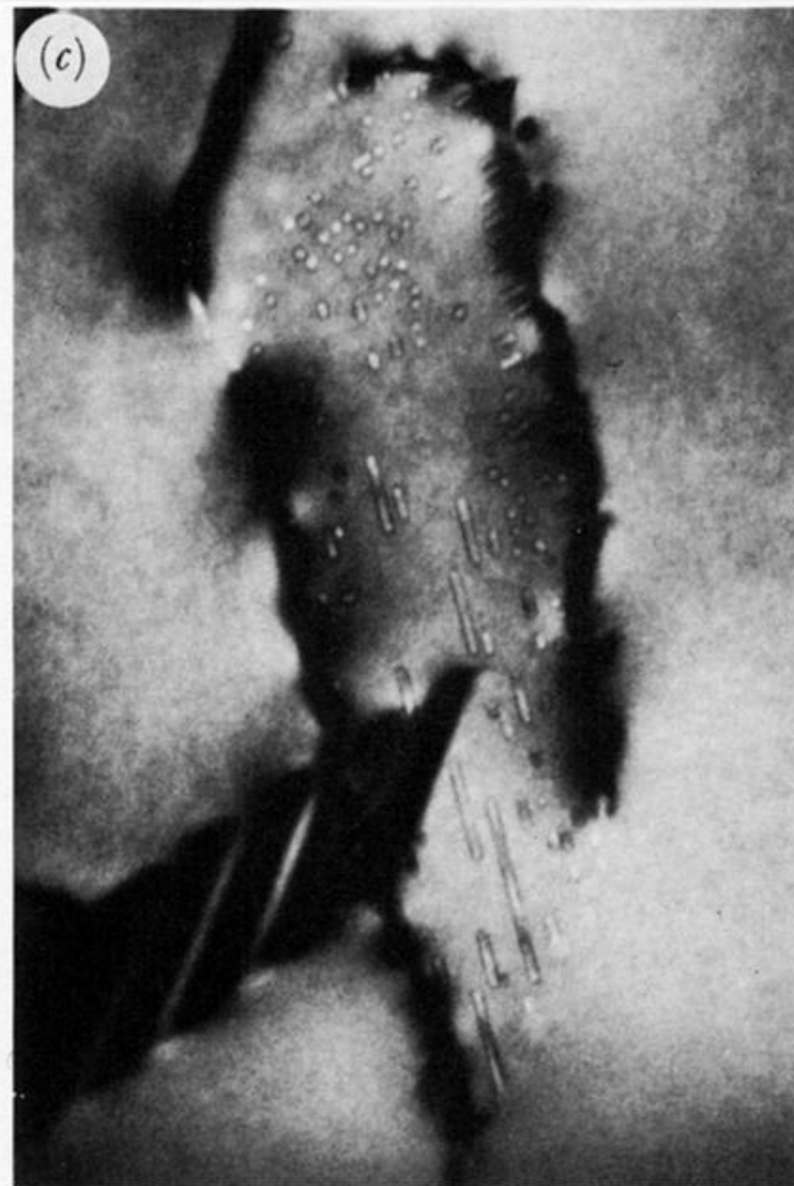
FIGURE 3. Detail in the large voidite-containing loop at the centre of the field of figure 2. The image is rotated about 17^\circ clockwise relative to figure 2 (magnification \times 160000 ). (a) Enlargement from the low-magnification micrograph, figure 2. (b) High magnification and resolution, electron accelerating voltage 200 kV, close to optimum focus. Longest voidite image is about 3 \times 80 nm in projection. (4709, original magnification \times 10^5 .) (c) As (b), but underfocused by about 1 \mu\text{m} (4716).
